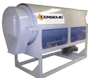
Continuous mixer of rotary drum type, with adjustable speed and inclination, with an input of the raw materials by one end and exit of the ready-mix by the other. Mix the dosed solid ingredients also continuously.
