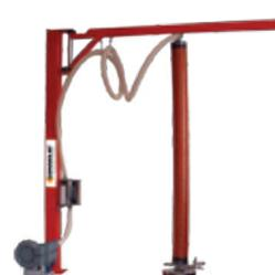
System for lifting and handling of loads developed to facilitate the action of stacking and unpacking of bags, boxes and other items with a flat surface, within the norms of safety and ergonomics for the handling of these packages.
