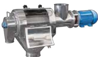
It has the function of sifting the product by swirling, effecting the separation without friction or pressure. The sieve basket can be fabricated or perforated steel sheets with the possibility of exchange without the need for special tools.
