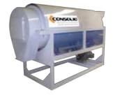
Continuous mixer of rotary drum type, with adjustable speed and inclination, with an input of the raw materials by one end and exit of the ready-mix by the other. Mix the dosed solid ingredients also continuously.
